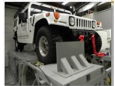
Figure 1. Vanderbilt’s frame integrity structural test fixture.
